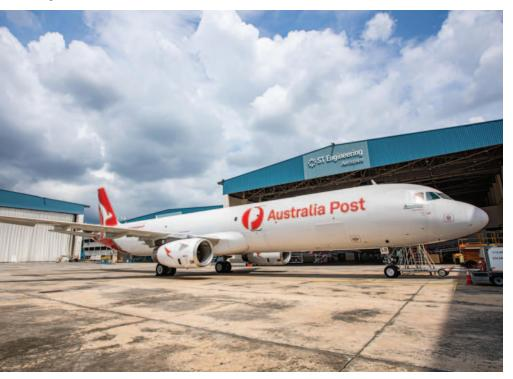
gross structural payload is about 28 tonnes or 61,729lbs, depending on the weight variant of the feedstock aircraft.
