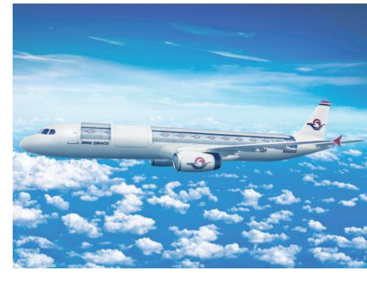
cargo capacity is unchanged at 1,270 cu ft. This gives the A321-200SDF a total volumetric capacity of 7,345 cu ft *(see table, page 48)*. Once the STC has been issued, the A321-200SDF is expected to achieve a gross structural payload up to 28.2 tonnes or 62,170lbs *(see table, page 48)*.
